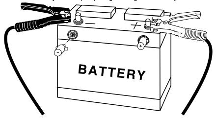
**Note!** Take special care when connecting to battery side terminals. If necessary use a side post adapter to prevent thread damage. When testing dual post batteries always connect load clamps to the post to which the system is attached. If a load test is made from a post connection and the alternator is mounted to side terminals a battery load test can be completed, but a continuity problem may still be in the side terminals when testing the alternator.
